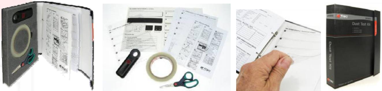
**Standards** The SP3200 Dust Test Kit follows the standard ISO8502-3 "Assessment of dust on steel surfaces prepared for painting (pressure-sensitive tape method)" and is also mentioned in the IMO-PSPC MSC.215(82) and MSC.244(83) resolutions.
