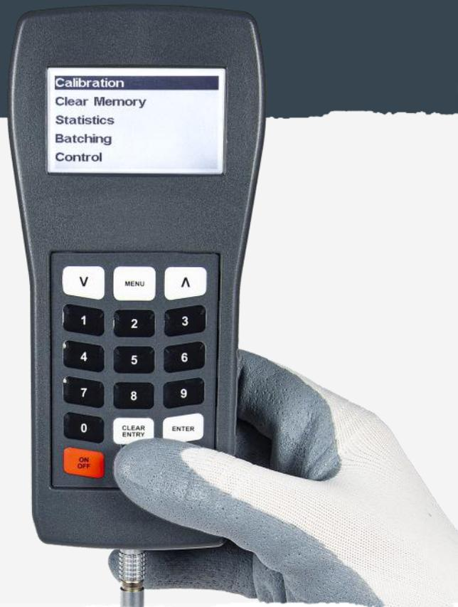
To exit from the menu, press the Menu button again and the Coating Thickness Meter will revert back to normal measurement mode.
