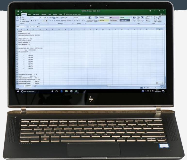
Connection is made using the optional USB PC Download Cable to the download socket on the Coating Thickness Meter and the USB port on the computer. Ensure the Coating Thickness Meter is switched off when connecting the cable.
